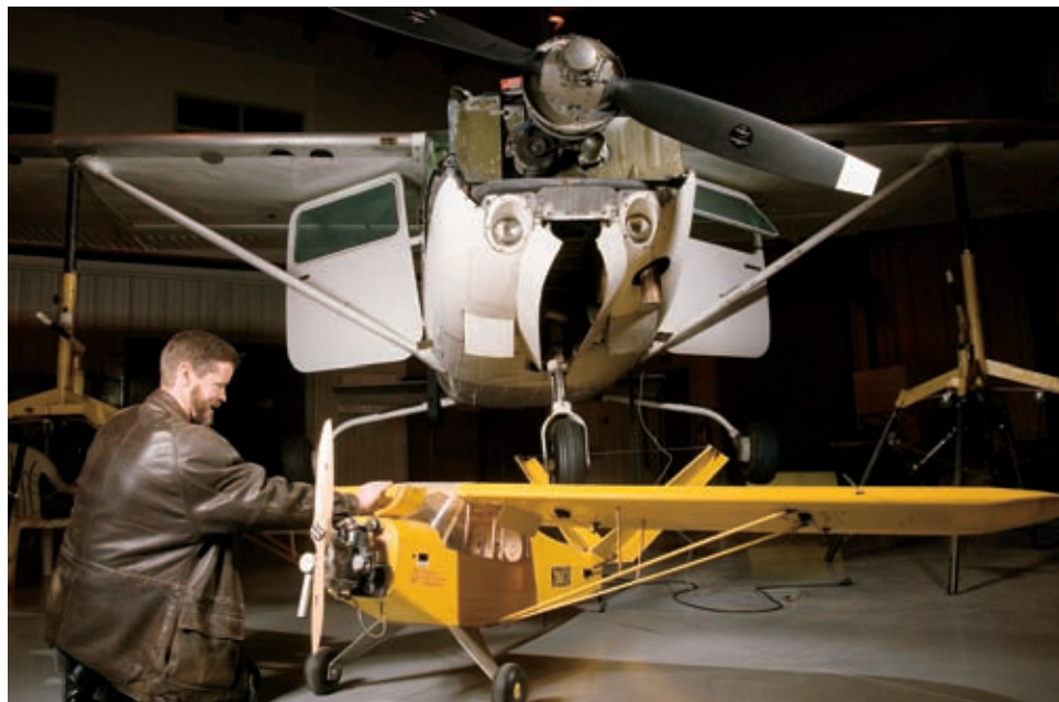
■ Associate Professor Rick Hale tinkers with a prototype aircraft built to test specific features of the Meridian, including its innovative V-tail. When built, the Meridian will be as large as the white airplane in the background above.
